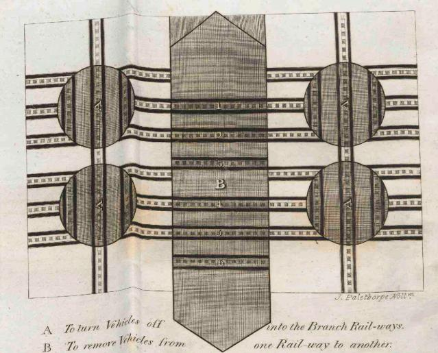
. The Rails on which the Vehrcles are to run being Convex and the Rim of the Carriage-Wheel Concave shew at one view the Ease, Security, and Velocity with which Vehicles may be impelled by Mechanic-power. The Cog-rail in the middle of each Rail-way 1.2.3.4.5.6. is solely for the operative power of the Cog-Wheel connected with the Steam-Engine.
