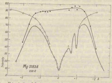
Fig. 1. — Determination of the inner part of the profile of a strong Fraunhofer line; exposure with narrow monochromator-slit in order to avoid scattered light and ghosts (first ghost at 3.5 A from principal line);
