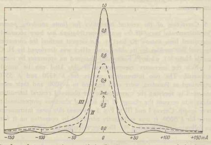
Fig. 3. — I: instrumental curve of the Potsdam grating spectrograph for  $\lambda$  5000; II: instrumental curve I transformed by the peak-function operation; I and II have equal areas;
